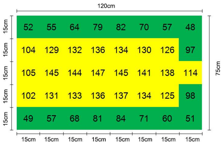
PPFD Map of GLTW050 at 40cm(hanging height) Test Footprint: 75cm x 120cm
